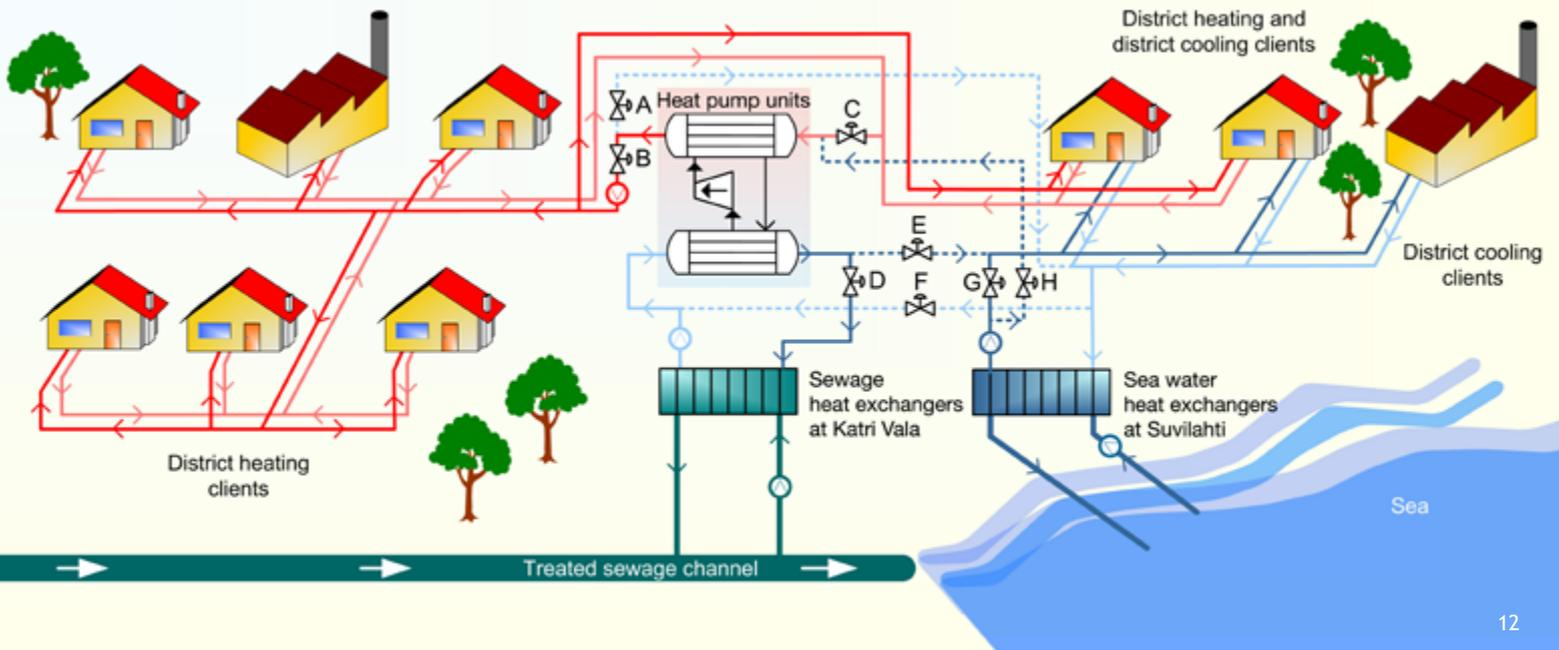
Thus, the Unitop® 50FY heat pumps are able to produce the full temperature lift required. The chilled water produced is absorbed completely by the district cooling system. During times without heat load, the condensing temperature is lowered to match with sea water conditions and the heating energy is rejected to the sea, resulting in a very high COP. (Valves A + H open, Valve B + C closed, Valves E + F open, Valves D + G closed).
